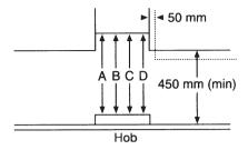
A: Built-in Electric Hob: 650mm clearance B: Built-in Gas Hob: 700mm clearance C: Slot-in Electric Cooker: 685mm clearance D: Slot-in Gas Cooker: 767mm clearance
